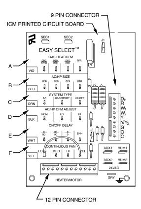
Fig. 8—Detail of SPP Printed-Circuit Board
